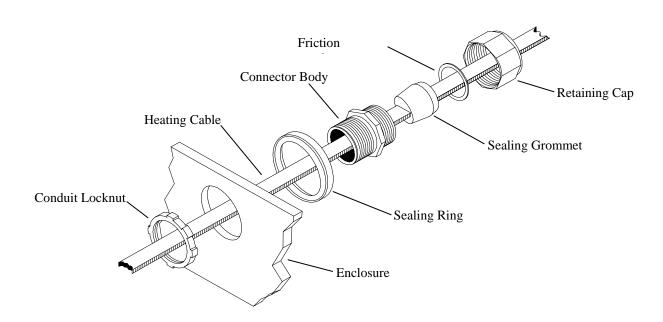
Note: This entry seal is suitable for use with any approved enclosure with a maximum wall thickness of .1875" or conduit outlet/junction box with .75" threaded hubs.
